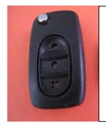
Do Not open remote. Gently remove an old rubber pad from your remote. Your remote should look like the one in the picture on the side, free of any old rubber pieces and dirt.
